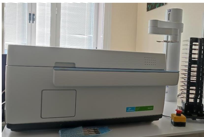
Figure 23. **Operetta system for high content imaging of lentivirus transduction efficiency**
