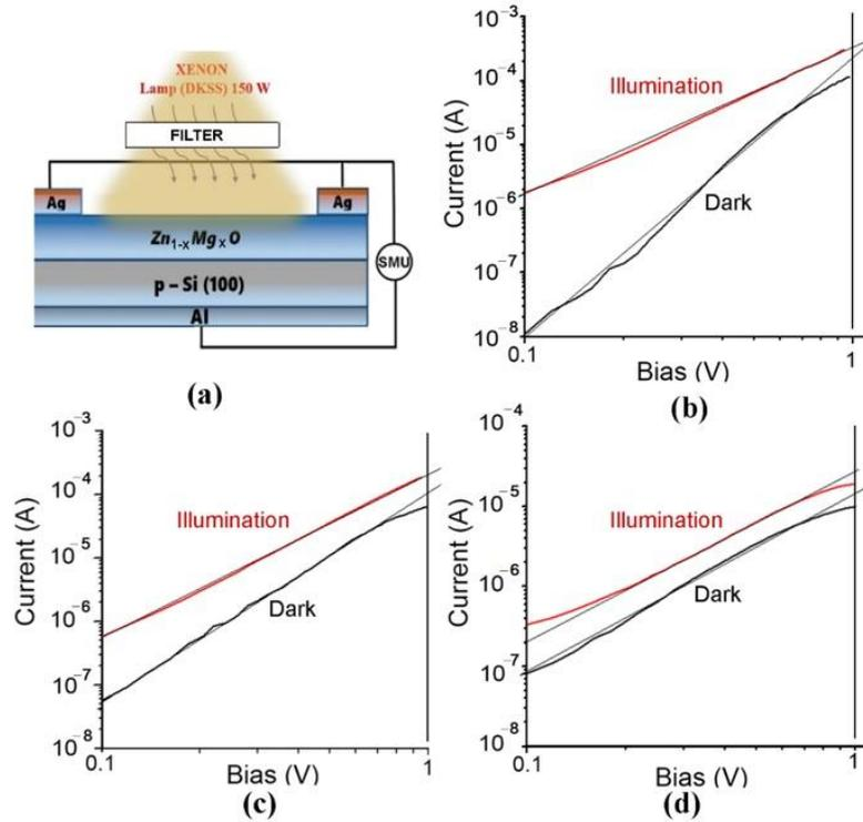
**Fig. 14. Design of an  $n\text{-Mg}_x\text{Zn}_{1-x}\text{O}/\text{p-Si}$  photodiode (a) and current-voltage characteristics of the devices plotted for double-logarithmic scale direct bias for  $x$  values of 0.1 (b), 0.2 (c) and 0.4 (d).**
