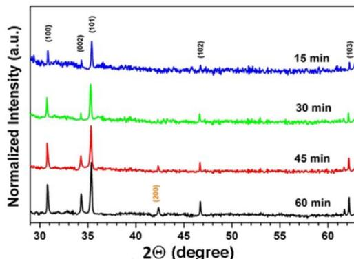
**Fig. 4. XRD pattern of Zn<sub>0.5</sub>Mg<sub>0.5</sub>O films deposited on Si substrate by spin coating method and subjected to thermal treatment in a combined atmosphere of (O<sub>2</sub> +Ar) at 500 °C for different process duration.**
