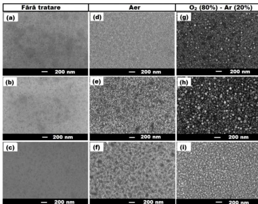
**Fig. 5. SEM images (top view) of Zn<sub>0.8</sub>Mg<sub>0.2</sub>O/Si oxide films obtained by the spin coating method and thermally treated in different atmospheres: I column - samples without heat treatment with 15, 10, 5 layers (a, b, c); II column - samples thermally treated in air with 15, 10, 5 layers (d, e, f); III column - samples thermally treated in atmosphere of (O<sub>2</sub> +Ar) with 15, 10, 5 layers (g, h, i).**
