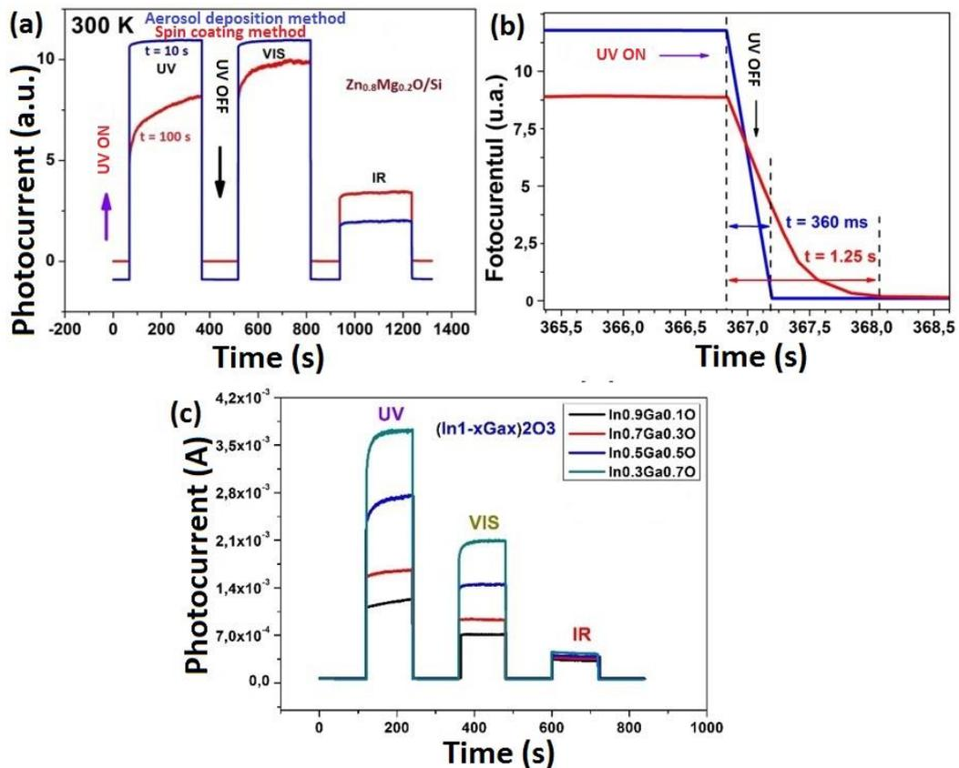
Fig. 13. Photocurrent relaxation measured at 300 K in vacuum under irradiation with different wavelengths for oxide films of  $Zn_{0.8}Mg_{0.2}O$  (a, b) and  $(Ga_xIn_{1-x})_2O_3$  (c).
