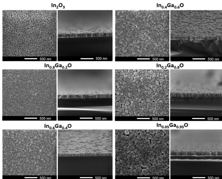
**Fig. 10.** SEM images (top view and cross section) of oxide films of  $(Ga_xIn_{1-x})_2O_3$  grown on Si substrates by aerosol deposition method.
