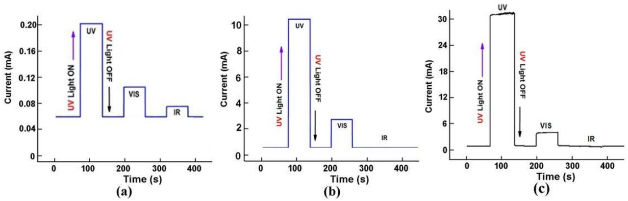
**Fig. 16.** Photocurrent relaxation measured at 300 K with irradiation at different wavelengths for a photodetector with a  $\text{Zn}_{0.80}\text{Mg}_{0.20}\text{O}$  film (a), a photodetector with  $n\text{-Zn}_{0.90}\text{Mg}_{0.10}\text{O}/n\text{-Zn}_{0.60}\text{Mg}_{0.40}\text{O}$  films (b) and a photodetector with  $n\text{-Zn}_{0.85}\text{Mg}_{0.15}\text{O}/n\text{-Zn}_{0.65}\text{Mg}_{0.35}\text{O}$  films (c).
