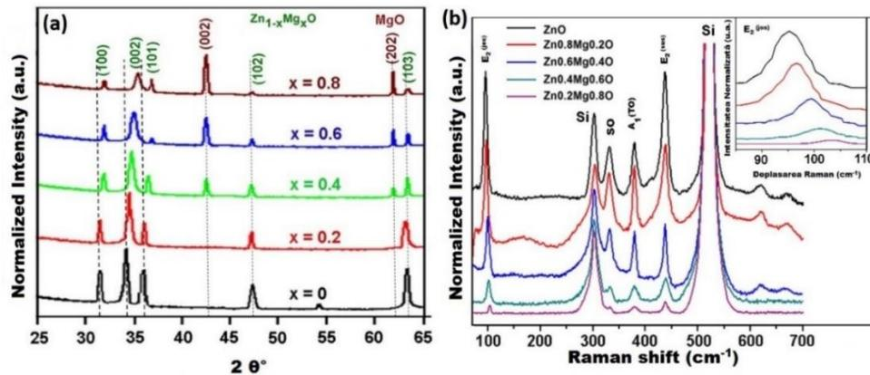
**Fig. 9.** XRD pattern (a) and RAMAN spectra (b) of  $Mg_xZn_{1-x}O$  films deposited on Si substrate by the aerosol deposition method.
