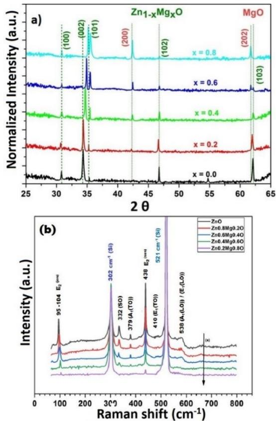
**Fig. 2.** XRD pattern (a) and Raman spectra (b) of  $\text{Mg}_x\text{Zn}_{1-x}\text{O}$  films deposited on Si substrate by the spin coating method
