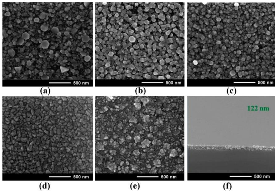
**Fig. 1. SEM images of  $Mg_xZn_{1-x}O$  films deposited on Si substrate by the spin coating method and thermal treated at 500 °C for 1 h in a combined atmosphere of ( $O_2 + Ar$ ). The  $x$ -values of the films are as follows: 0 (a); 0.2 (b); 0.4 (c); 0.6 (d); 0.8 (e). The SEM image in cross-section of a film with  $x = 0.4$  is shown in (f)**
