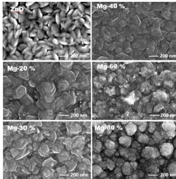
**Fig. 8. SEM images (top view) of oxide films of  $Mg_xZn_{1-x}O$  with the composition range of  $x = 0.00 - 0.80$  deposited on Si substrates by aerosol deposition method.**
