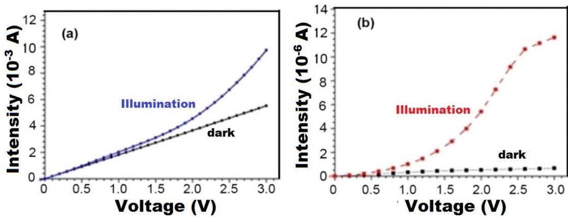
Fig. 12. Current-voltage characteristics in the dark and under UV light irradiation for  $Zn_{0.8}Mg_{0.2}O$  films deposited on Si Substrate by aerosol deposition (a) and by spin coating (b).
