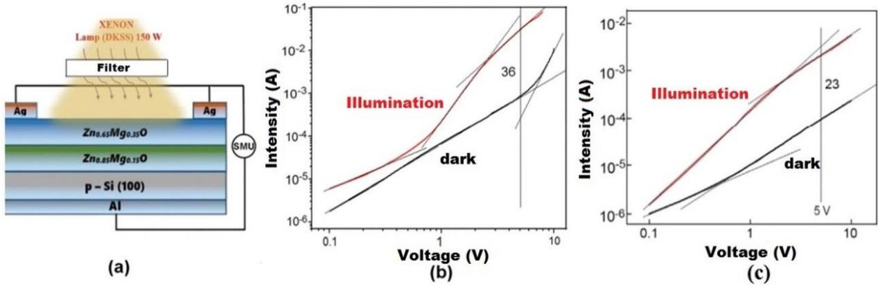
**Fig. 15. (a) Design of an Al/p-Si/n-Zn<sub>0.85</sub>Mg<sub>0.15</sub>O/n-Zn<sub>0.65</sub>Mg<sub>0.35</sub>O/Ag photodiode. (b) Current-voltage characteristics of the device fabricated by aerosol deposition method, plotted for double-logarithmic scale direct bias at forward (a) and reverse (b) bias voltages.**
