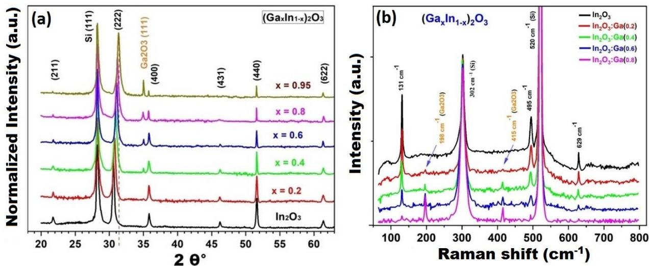
**Fig. 11. XRD pattern (a) and RAMAN spectra (b) of  $(\text{Ga}_x\text{In}_{1-x})_2\text{O}_3$  films deposited on Si substrate by the aerosol deposition method.**
