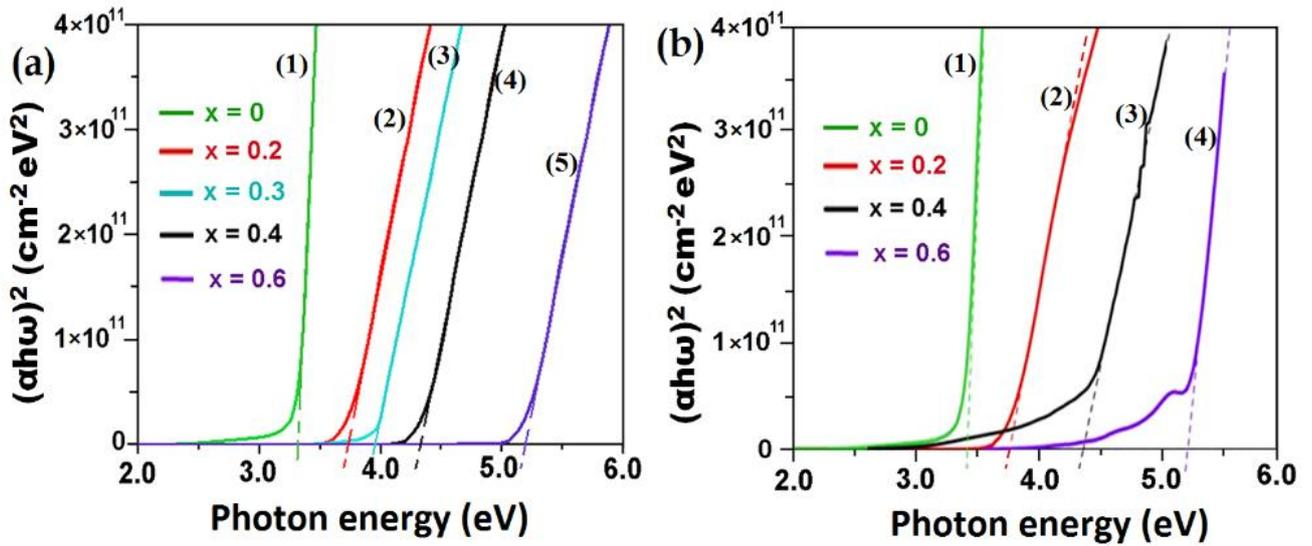
**Fig. 17.** Tauc plot of optical absorption spectra measured at room temperature for  $\text{Mg}_x\text{Zn}_{1-x}\text{O}$  films deposited on quartz substrates by spin coating (a) and aerosol deposition method (b).
