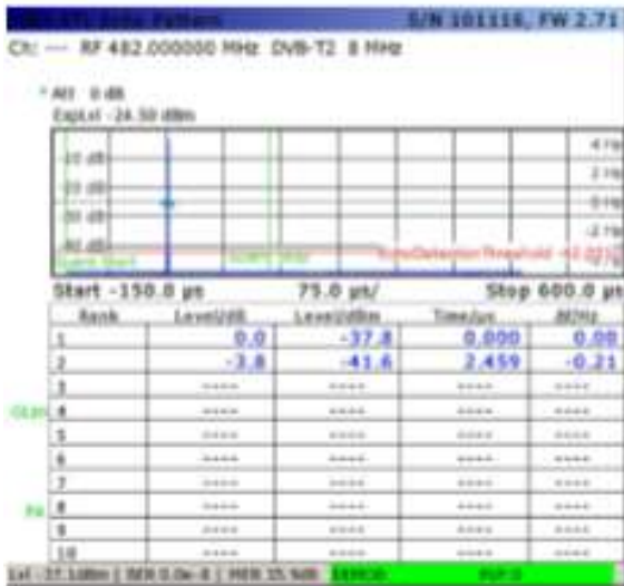
Fig. 3.8. Parametrii semnalului DVB-T2 SFN SISO: Time offset 2 \mu s; Level (- 37.1 dBm); \Delta Level (3.8 dB), Amplitude 14.04 dB; Phase 85.29 deg; MER(f); MER (PLP, rms) 33.9 dB
