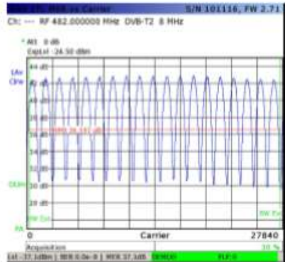
Fig. 3.8. Parametrii semnalului DVB-T2 SFN SISO: Time offset 2 \mu s; Level (- 37.1 dBm); \Delta Level (3.8 dB), Amplitude 14.04 dB; Phase 85.29 deg; MER(f); MER (PLP, rms) 33.9 dB
