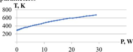
**Fig. 4.8. The dependence of the cathode temperature on the power dissipated on it from the current source [38]**
