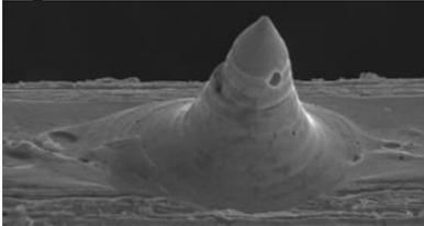
**Fig. 4.1. The component parts of the conical asperity: conical tip, truncated cone, and crater area**
