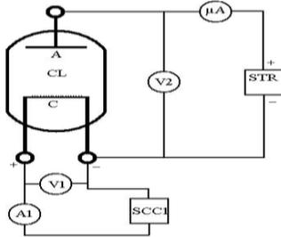
**Fig. 2.2. The main electrical diagram for determining the volt-ampere characteristics:**
