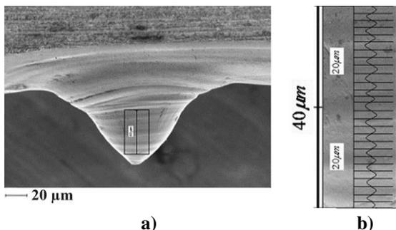
**Fig. 4.4. Surface morphology of the Taylor cone asperities: a) image obtained by the SEM method; b) determining the average wavelength for the transverse wave [18]**
