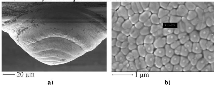
**Fig. 3.4. The lateral surface of the asperity [15]: a) presence of concentric waves; b) the presence of mosaic blocks on the lateral surface of the conical asperity**
