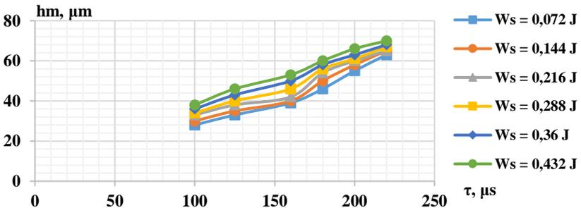
**Fig. 3.3. Dependence of the height of the menisci as a function of the duration of the discharge pulse**
