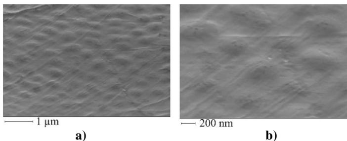
**Fig. 4.3. Micro- and nanometer-sized “undulations” are presented on the lateral surface of the conical asperities**
