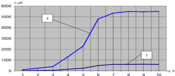
**Fig. 4.6. Emission volt-ampere characteristic obtained under express conditions, in which the potential difference between the cathodes remained a constant value [37]**
