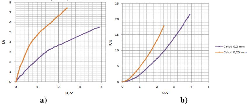
**Fig. 4.7. The volt-ampere characteristic (a) and the dependence of the power dissipated on the cathode (b) depending on the voltage applied from the power source for cathodes with diameters of 0.2 mm and 0.25 mm, respectively, made of tungsten alloy with 10%Re [38]**
