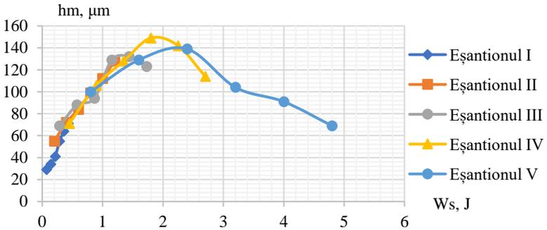
**Fig. 3.2. The dependence of the height of the menisci according to the energy released in the interstice.**
