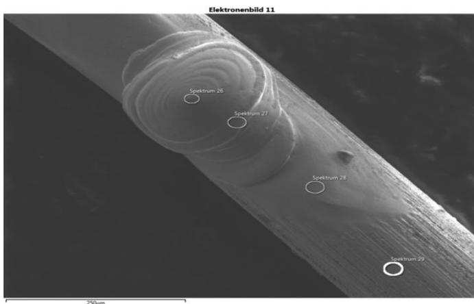
**Fig. 3.6. EDX analysis performed in four different areas of the sample- electrode**
