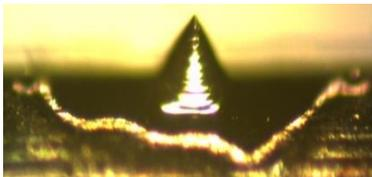
**Fig. 3.1. General view of the Taylor cone extracted by the EID method (height  $\approx$  60  $\mu$ m and the diameter of the base of this meniscus is of the order of 80  $\mu$ m)**
