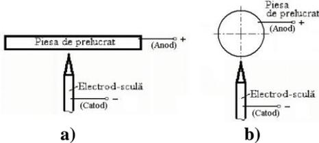
**Fig. 2.1. Schemes of positioning the electrodes used in the process of experimental research and their connection in the discharge circuit of the power pulse generator: a) flat sample case; b) cylindric sample case**
