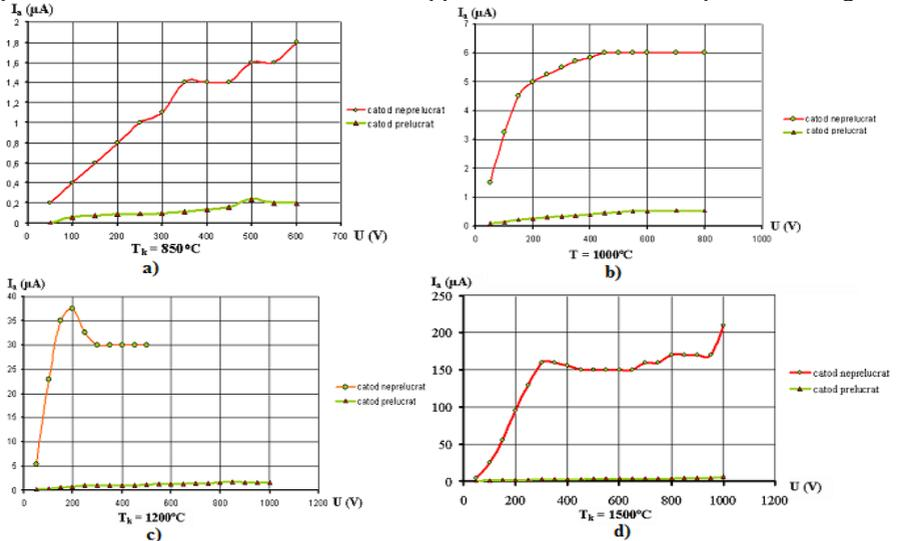
**Fig. 4.5. The volt-ampere characteristics obtained in express conditions, of the simple cathodes compared to those that were processed with the application of EID in air environment and that were not subjected to the process of deoxidation of the active surfaces: a)  $T_k = 850^\circ\text{C}$ ; b)  $T_k = 1000^\circ\text{C}$ ; c)  $T_k = 1200^\circ\text{C}$ ; d)  $T_k = 1500^\circ\text{C}$**
