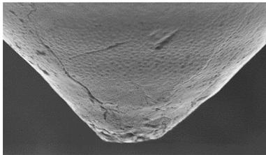
**Fig. 4.2. SEM image of the side surface of the tip of the conical asperity with the tip radius**
