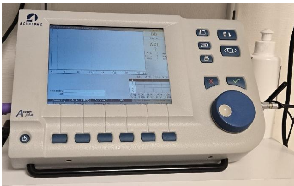
Fig. 2.11. Biometrul optic Ascan plus, Accutome, SUA.
