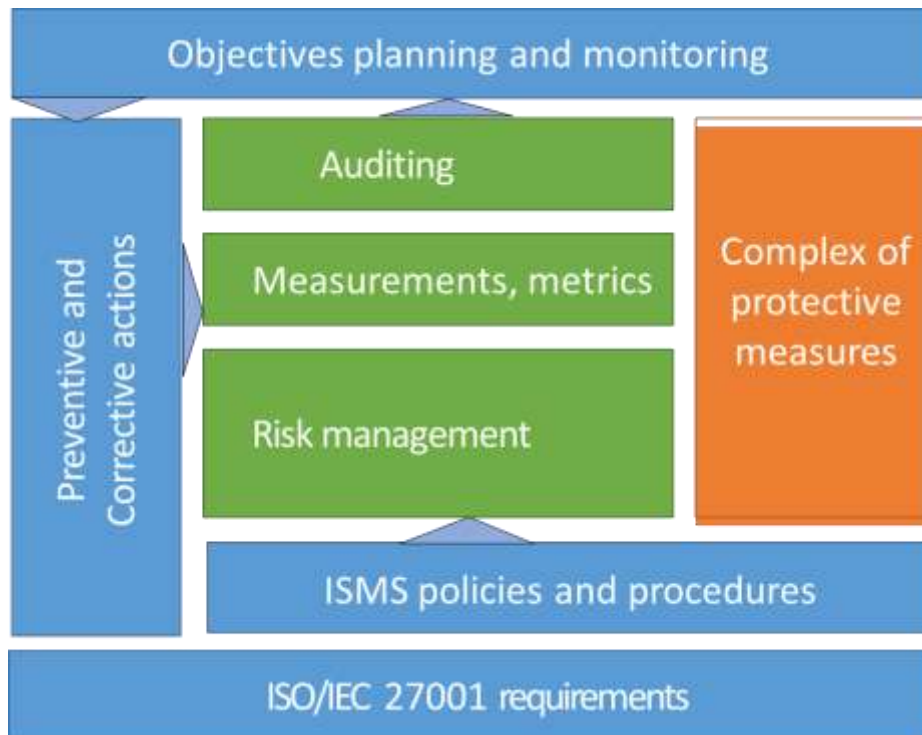
Figure 1. Main ISMS components and logic operation
